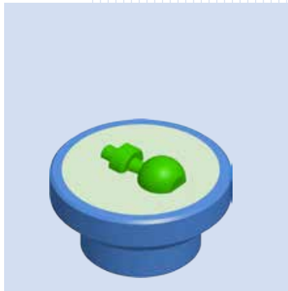
Knetharz aushärten lassen Harden the compound resin
