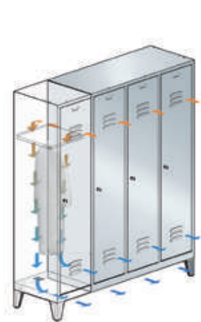
Ventilation concept The air outlet at the back of the cabinet base ensures good ventilation and drying in the compartment. In the case of base-mounted cabinets, ventilation is provided via openings above the recessed base.
